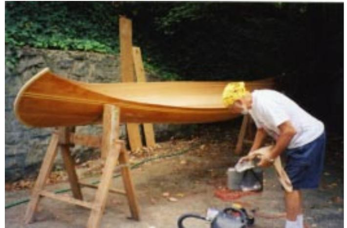
Left, the almost-completed stripper coming together along the keel. Above, building a stripper takes "some serious sanding." Below, the end: the finished and loaded stripper at a lunch stop on Holmes Creek. Photo above by Barb Reeves; photos left and below by The Hawk.
