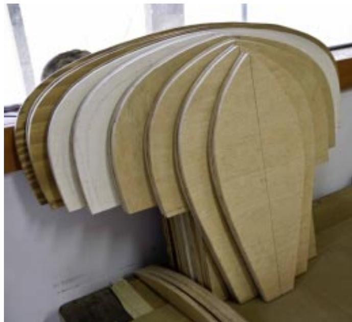
pieces of plywood and cut out the cross sections. Then I fished some 2x4's out of the basement, stuck plywood on top to make a 17 foot strong back and fixed the cross sections to it. This step is critical because if things aren't perfectly aligned your boat will look funny and will likely paddle crooked.
